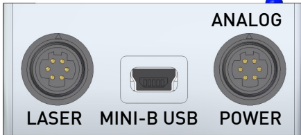
Figure: MX2 USB 2.0 and Analog interface
