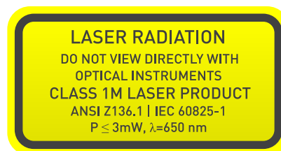
Image 16: Class 1M Laser safety label
